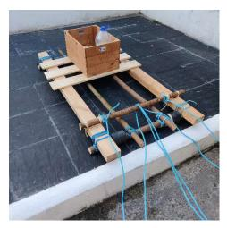
Rollers should go on a spar underneath the sled to help it roll on hard ground.
